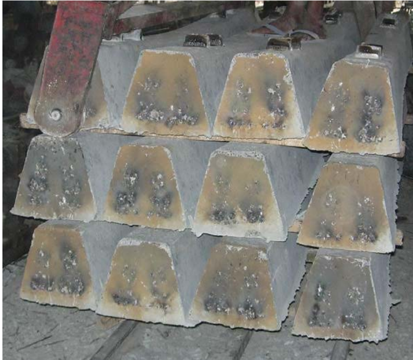
Figure: End of pre-tensioned railway sleepers
